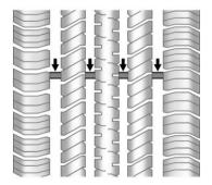
One way to tell when it is time for new tires is to check the treadwear indicators, which appear when the tires have only 1.6 mm (1/16 in) or less of tread remaining.
